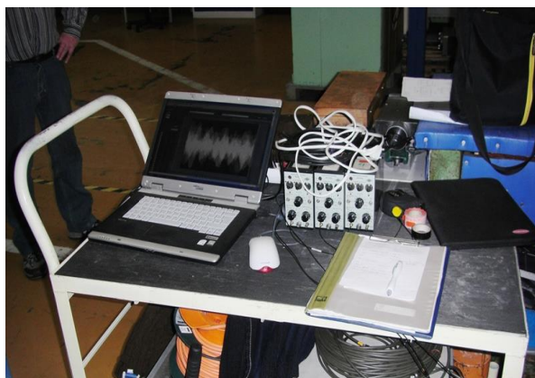
Fig. 1: Set of accelerometers with amplifiers and measuring PC in acquisition configuration to measure floor and mounts vibrations of the CNC lathe MORI SEIKI SL–204 (BK4).
