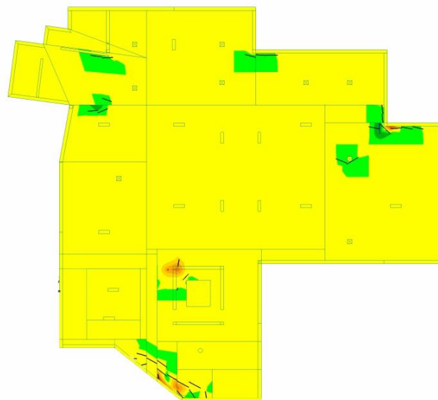
Fig. 2: Formation and development of cracks in a reinforced concrete slab with adapted material characteristics - equivalent height of water column 3.5 m, max. crack width 0.1 mm.
