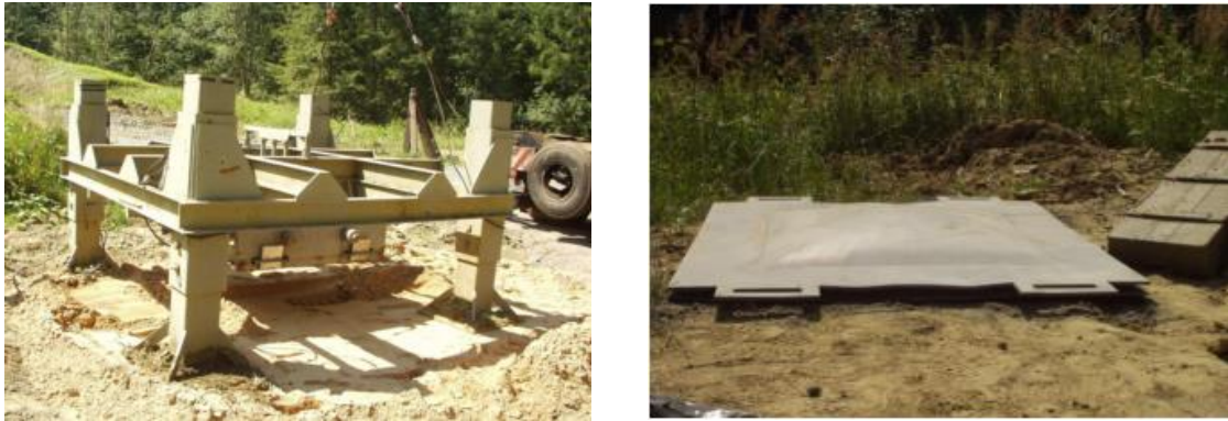
Fig. 1: Experimental equipment – stand and testing plate.
