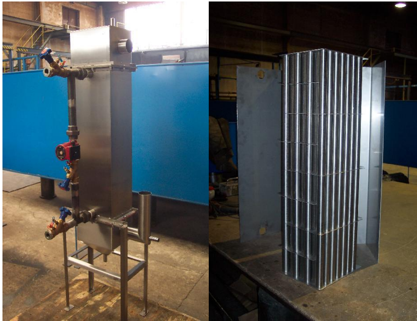
Fig. 1: Vertical shell-and-tube condenser.
