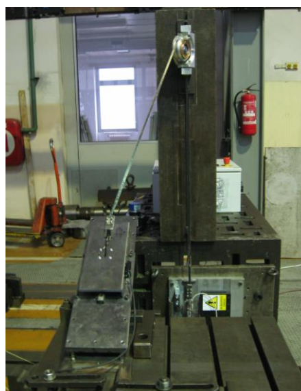
Fig. 1: Scheme and a real weight-fibre-pulley-drive mechanical system (asymmetric position of the weight).
