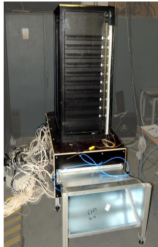
Fig. 3: Measurement of the mass flow rate in data rack using the pressure drop measurement across the nozzle.
