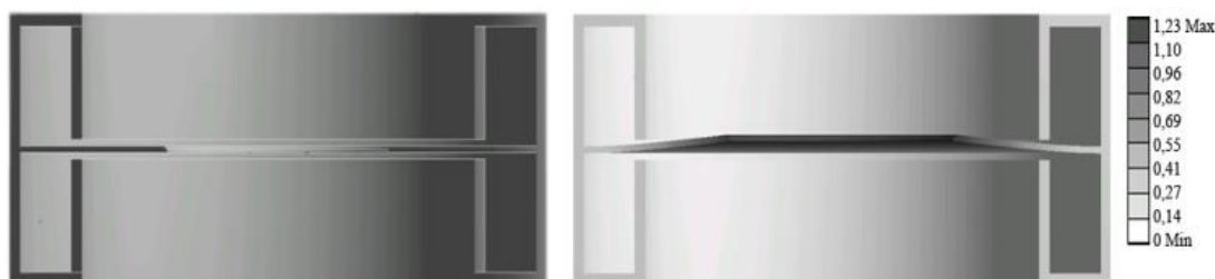
Fig. 1: Cut through undeformed and deformed model of the orifice plate ( \Delta p = 50 \text{ kPa} , t = 10 \text{ mm} ).
