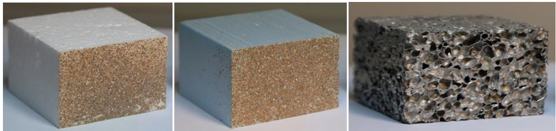
Fig. 1: Samples for impact tests – polystyrene, extruded polystyrene foam, Alporas foam (left to right).
