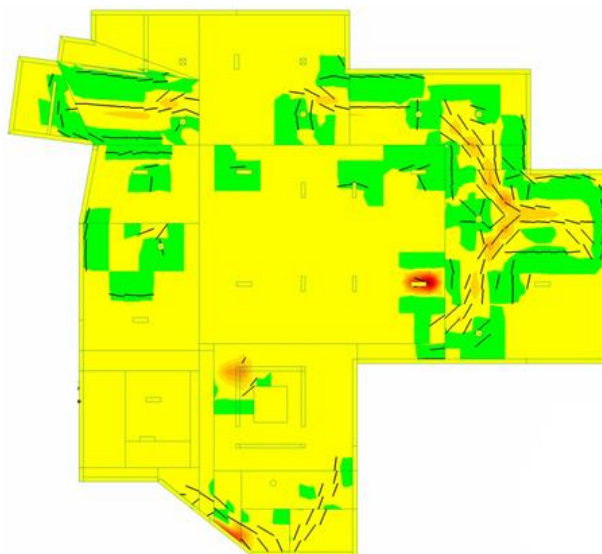
Fig. 1: Formation and development of cracks in a reinforced concrete slab - equivalent height of water column 3.5 m, max. crack width 0.295 mm.
