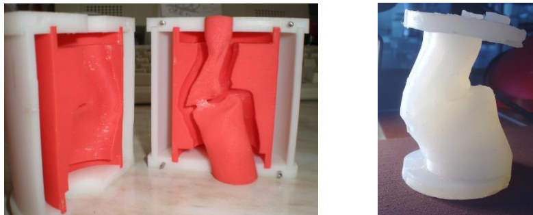
Fig. 1: The mould produced by 3D-printing and the casted larynx model made of silicone rubber.
