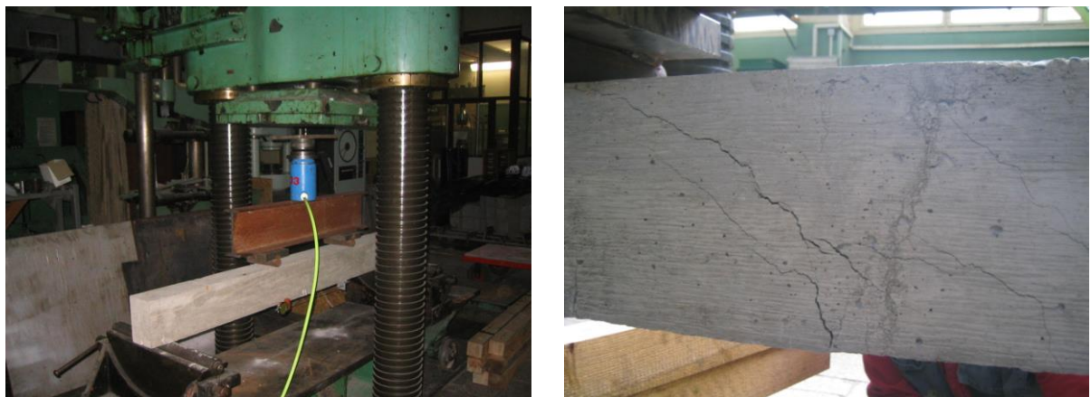
Fig. 3: Pictures experimental element, respectively. Detail the damaged beam.
