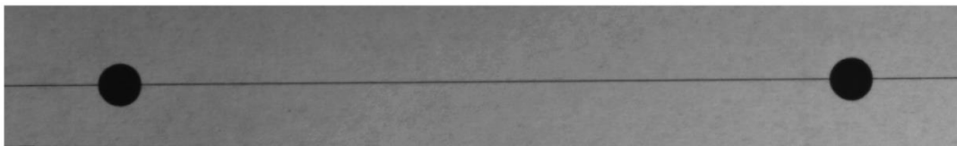
Fig. 2: Picture of the targets recorded by the high frequency camera with the points P1 (right), P2 (left).
