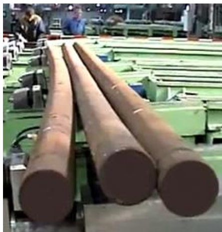
Fig. 1: Bars before straightening.
