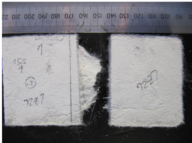
Fig. 4: Shear failure of the specimen.
