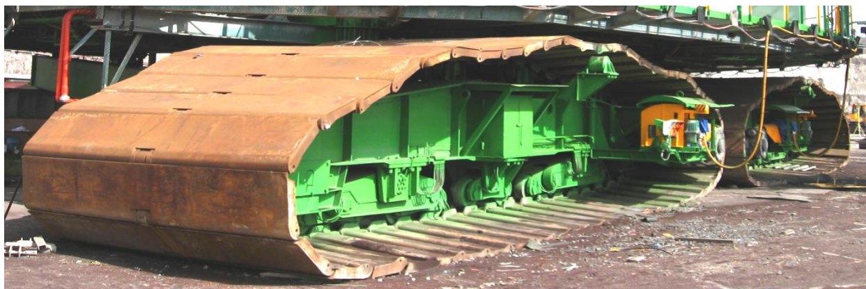
Fig. 1: A set of 2 caterpillar undercarriages. Source: author's archive.
