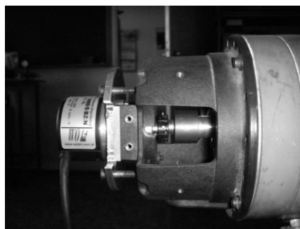
Fig. 4: Encoder with interface system placed on motor axis.
