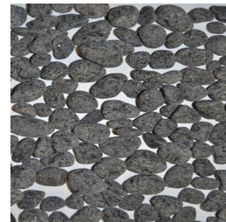
Fig. 2: The used material, graded basalt pebbles.
